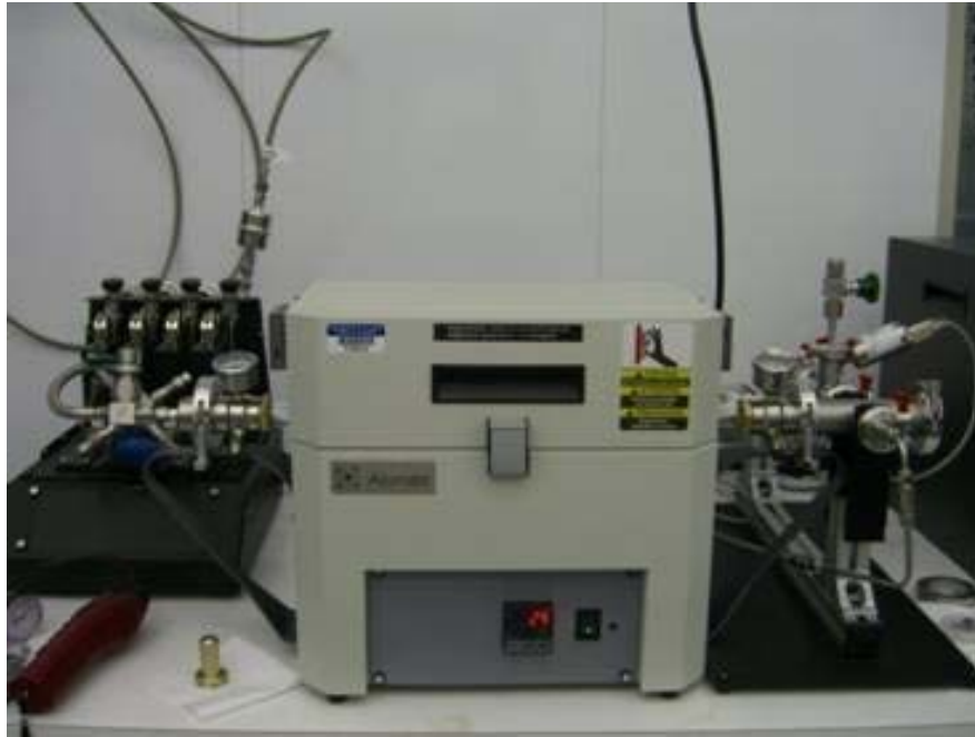
Figure 2.1: Photograph of the Atomate® carbon nanotube chemical vapor deposition reactor used in this study.
