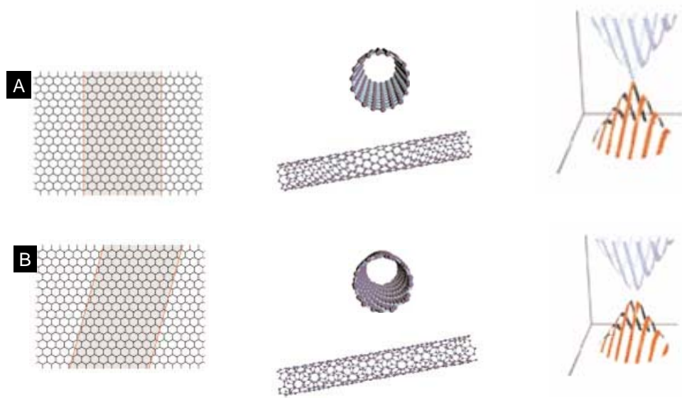
Figure 1.8: The left column shows a graphene sheet and the area that is rolled up to form a nanotube. The middle column shows the subsequent SWNT produced. The right column shows the energy states that are cut off by the nanotube with (A) no rolling angle and (B) an arbitrary rolling angle [11].
